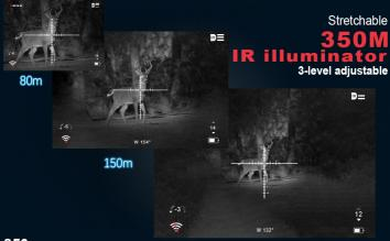
**850nm** provides long detective range with high sensitivity **940nm** evades recognition of animal with invisible light
